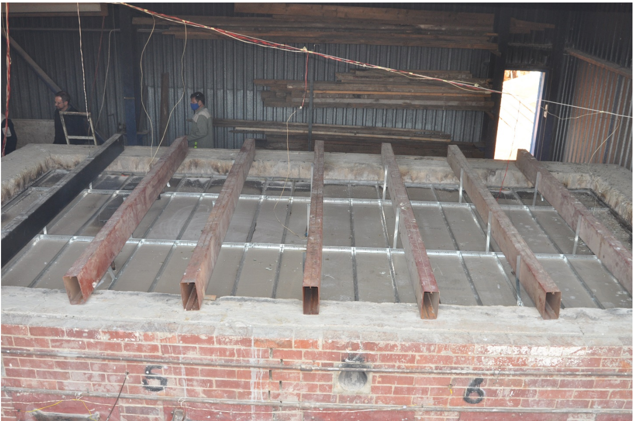
Figure 3.8: Unexposed side of specimen after conclusion of the test
