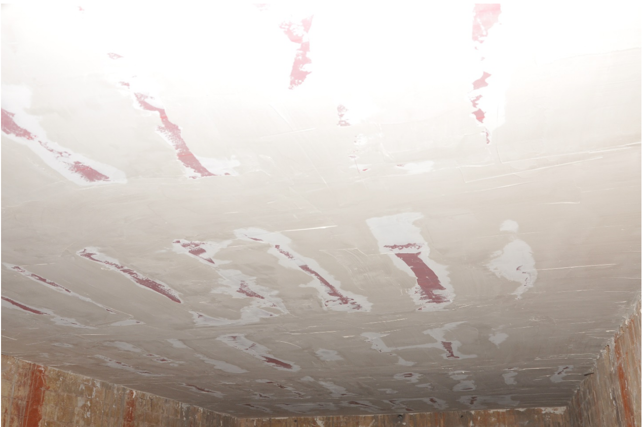
Figure 1.2: The FireShield Ceiling system from the exposed side
