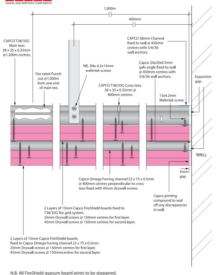
Board joints to be fitted and flushed with Capco jointing compound. Only final layer to be fitted with 50mm wide fibre-tape.
