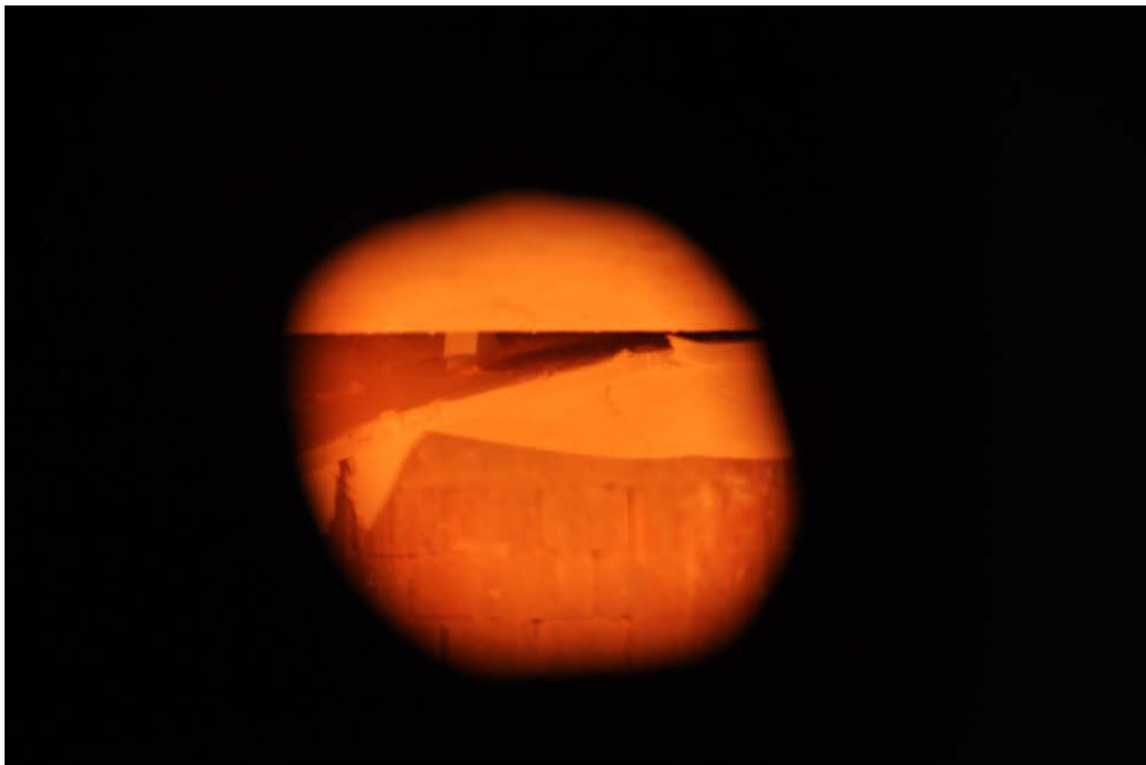
Figure 3.7: First layer of boards sagging significantly
