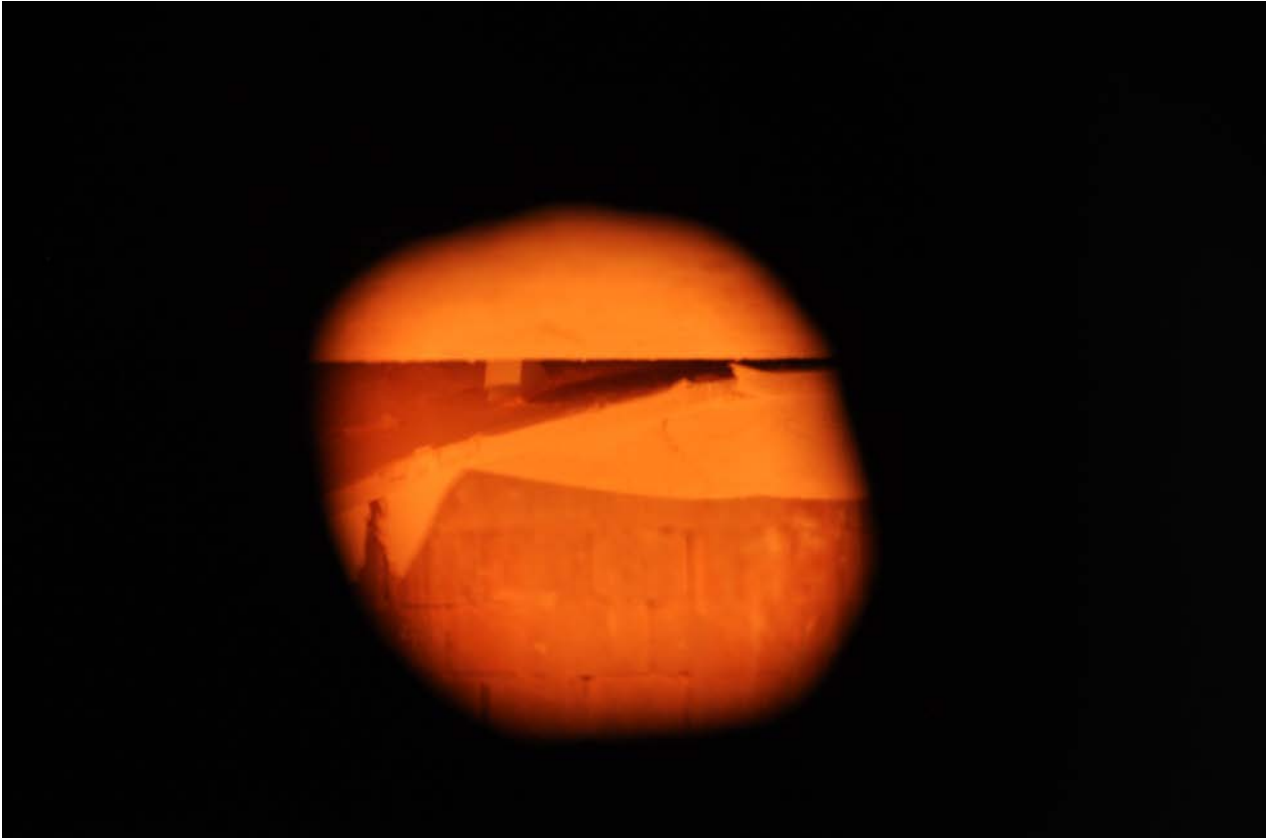
Figure 3.7: First layer of boards sagging significantly
